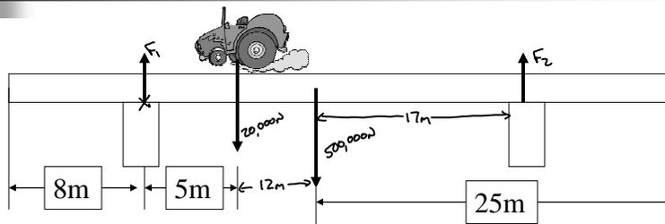
$$(20,000\text{N})(5\text{m}) + (500,000\text{N})(17\text{m}) - F_2(34\text{m}) = 0$$
