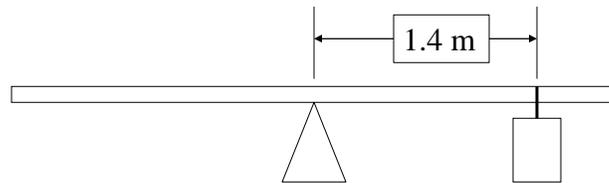
$$\tau = Fr = (5.3\text{kg})(9.8\frac{\text{m}}{\text{s}^2})(1.4\text{m}) = 72.7\text{N} \cdot \text{m}$$
